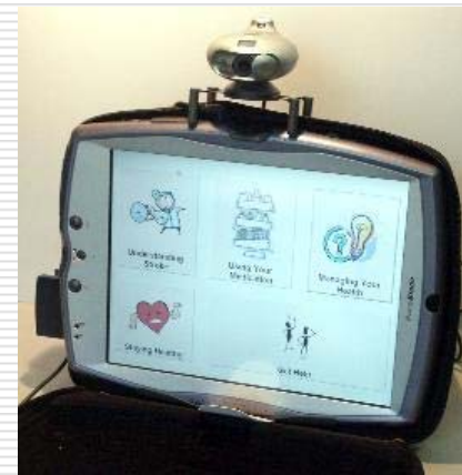
Prototype of the SMART Appliance based on a TabletPC showing touch-screen interface, Webcam, and wireless adapter.
